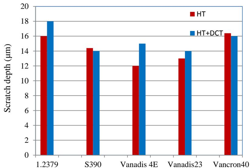
Fig 4-12: Results of scratch tests on flat samples
