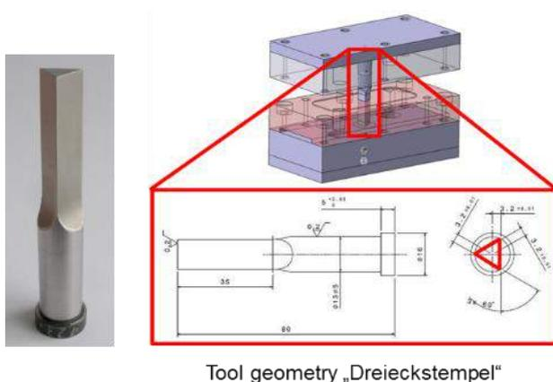
Figure 4-52: Used tool geometry and press for the lab scale tests
