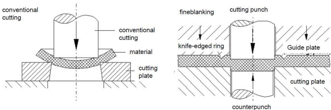
Figure 4-1: cutting technologies (left conventional cutting, right: fine blanking)
