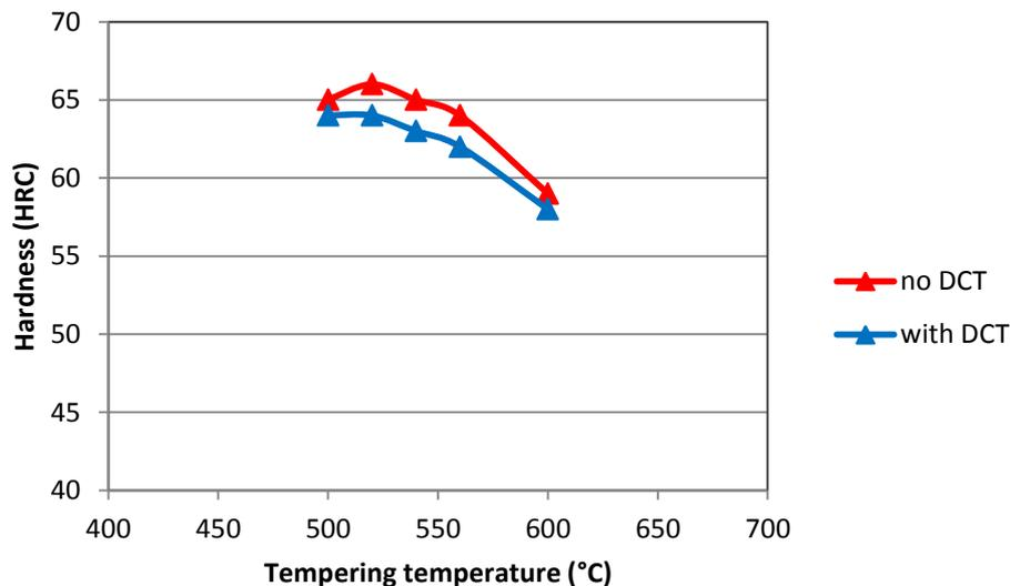
*Figure 4-9: Tempering diagram of Vancron 40*
