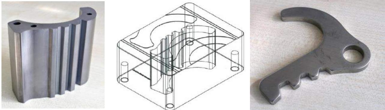
Figure 4-6: Tool geometry and work piece for fine blanking tests by company Meteor, “Mitnehmer”
