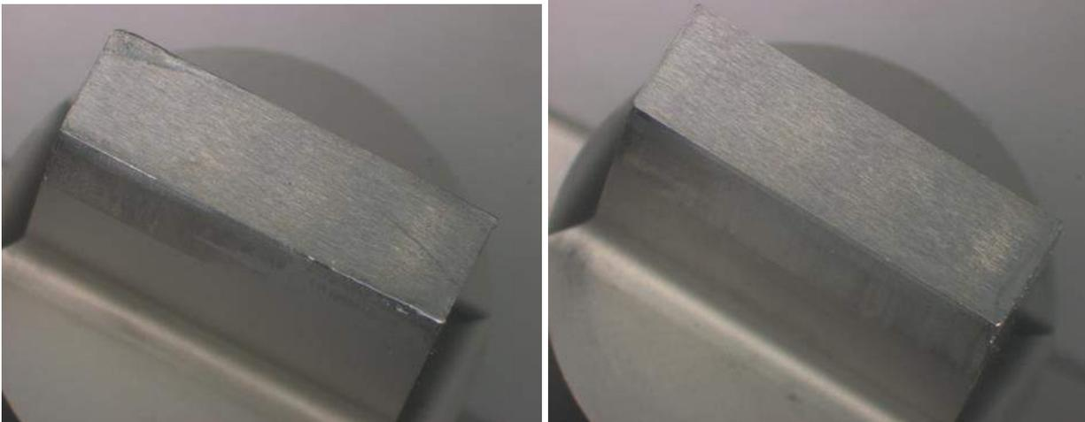
Figure 4-62: Detail of the punch HT (left) after 8500 strokes and the punch HT+DCT (right) after 10000 strokes
