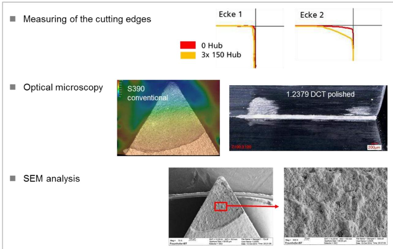
Figure 4-36: Used methods for wear analysis of the cutting tools after testing on laboratory scale.
