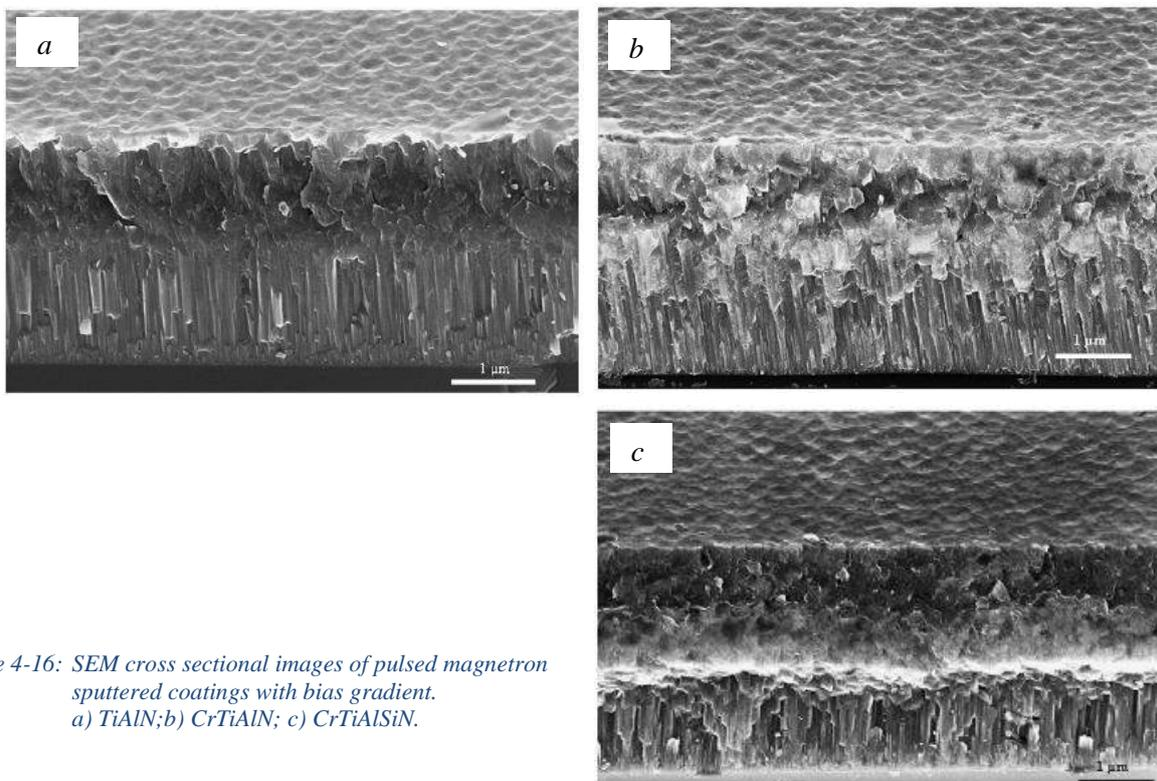
Figure 4-16: SEM cross sectional images of pulsed magnetron sputtered coatings with bias gradient. a) TiAlN; b) CrTiAlN; c) CrTiAlSiN.
