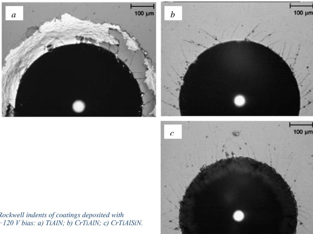
Figure 4-18: Rockwell indents of coatings deposited with  $-120\text{ V}$  bias: a) TiAlN; b) CrTiAlN; c) CrTiAlSiN.
