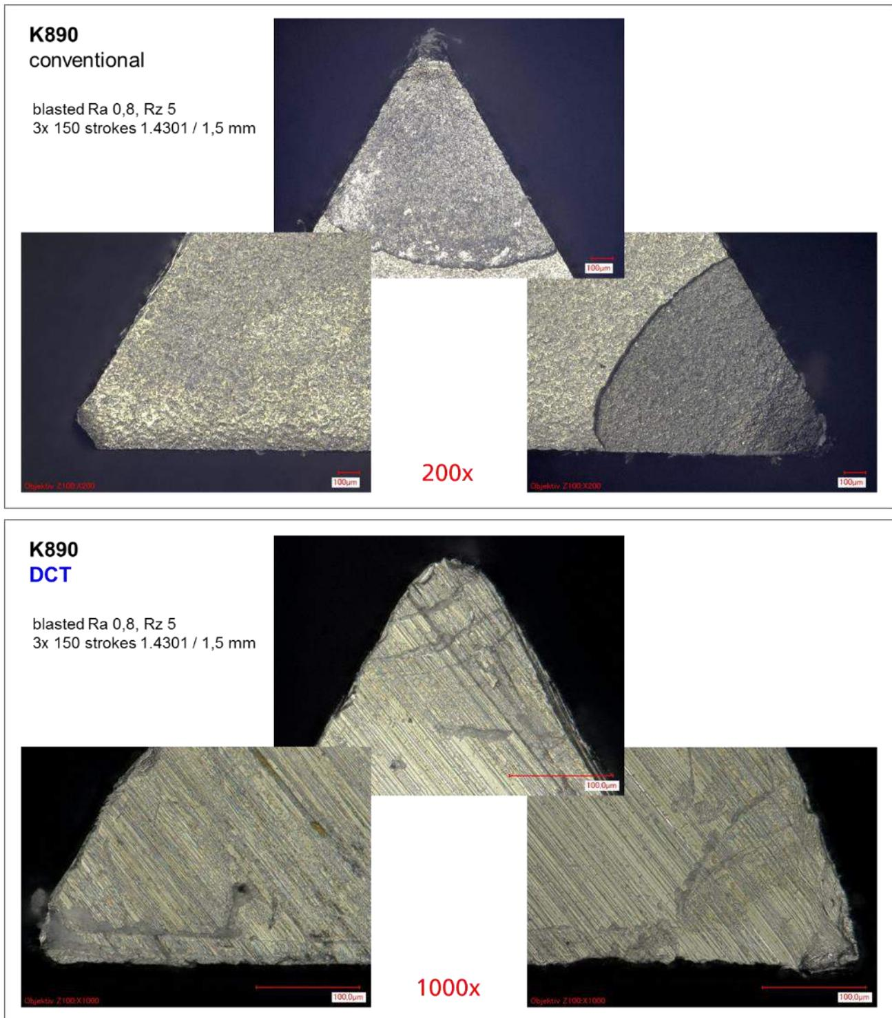
Figure 4-40: Comparison of the wear at the cutting edges of conventional and DCT treated K890 examined by optical microscopy.
