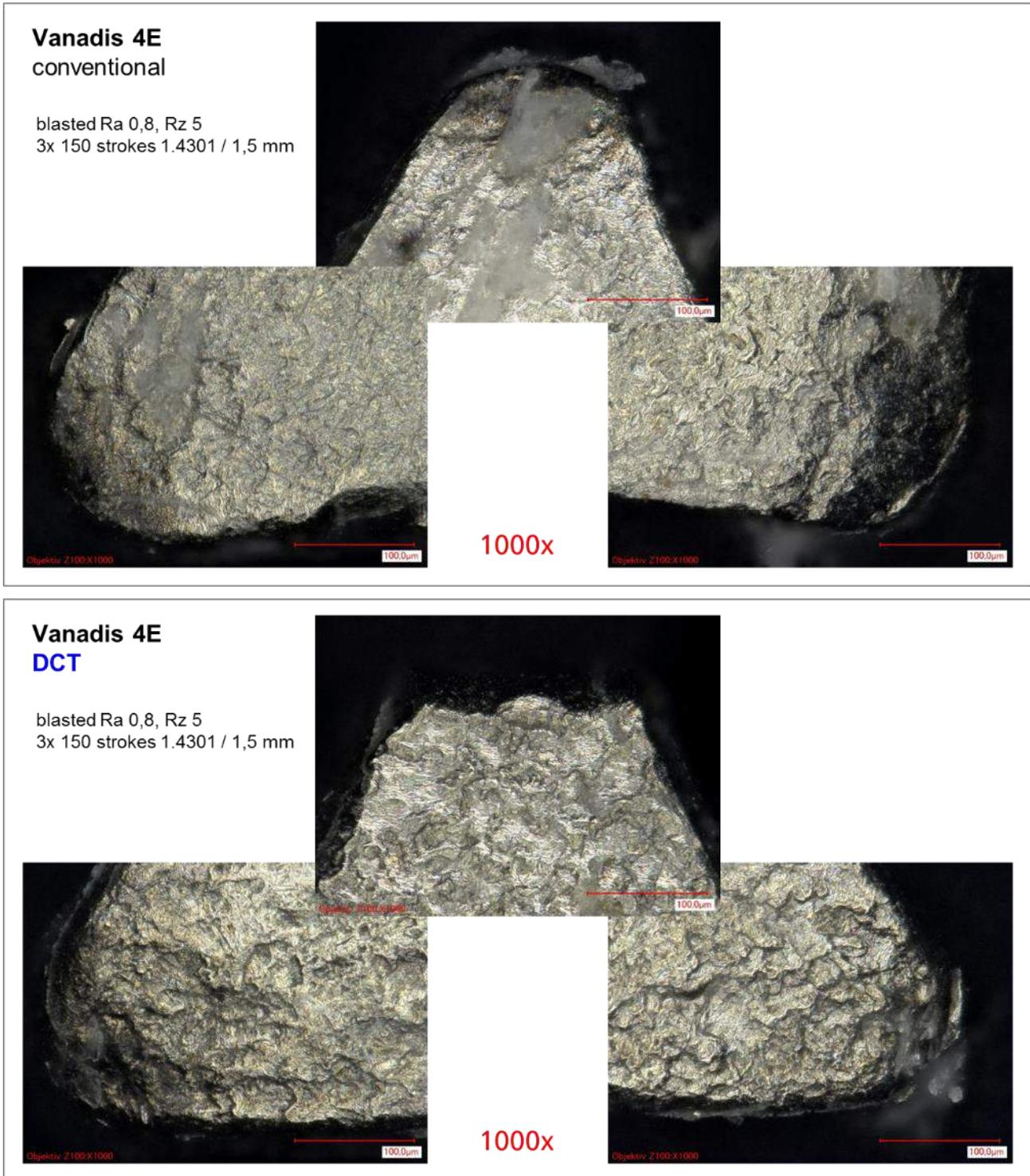
Figure 4-42: Comparison of the wear at the cutting edges of conventional and DCT treated Vanadis 4E examined by optical microscopy.
