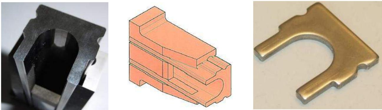
Figure 4-5: Tool geometry and work piece for blanking tests by company Karl Naumann GmbH, “gear folk”
