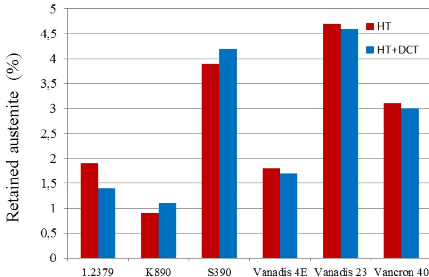
Figure 4-10: Retained austenite after heat treatment
