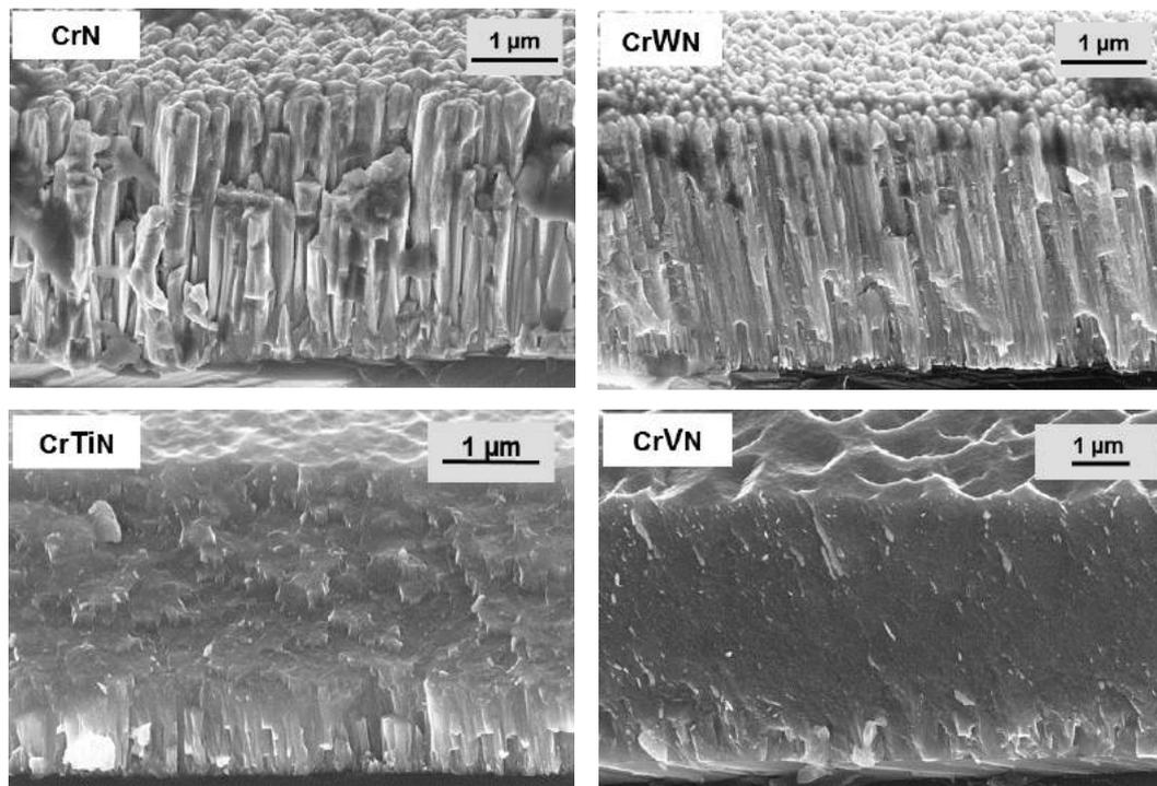
*Figure 4-19: SEM cross sectional images of different magnetron sputtered coatings, DC substrate bias – 200 V, Cr 6 kW.*
