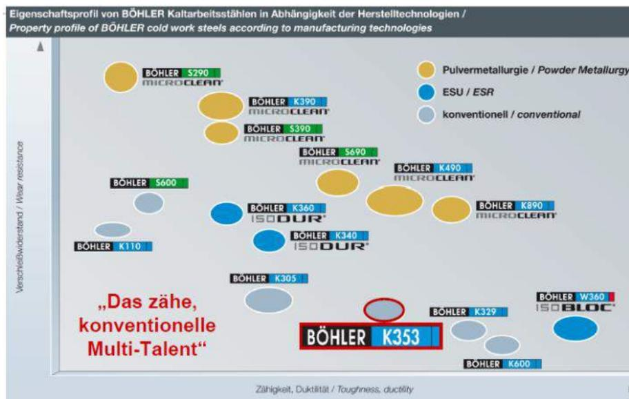
Figure 4-7: Performance of tool steels according to Böhler
