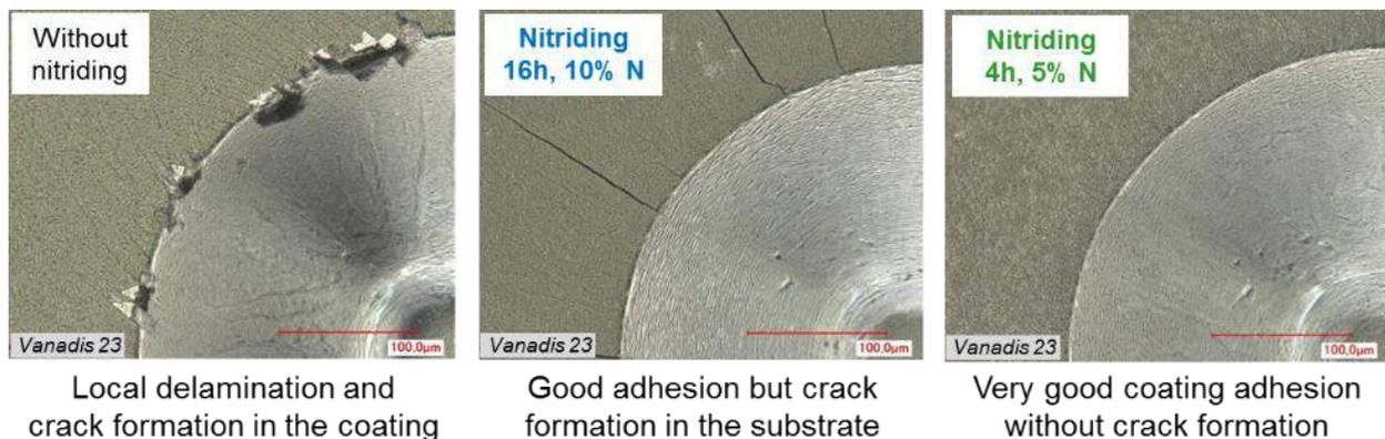
Figure 4-32: Influence of the nitriding treatment on the coating adhesion and load bearing capacity of CrVN on Vanadis 23.
