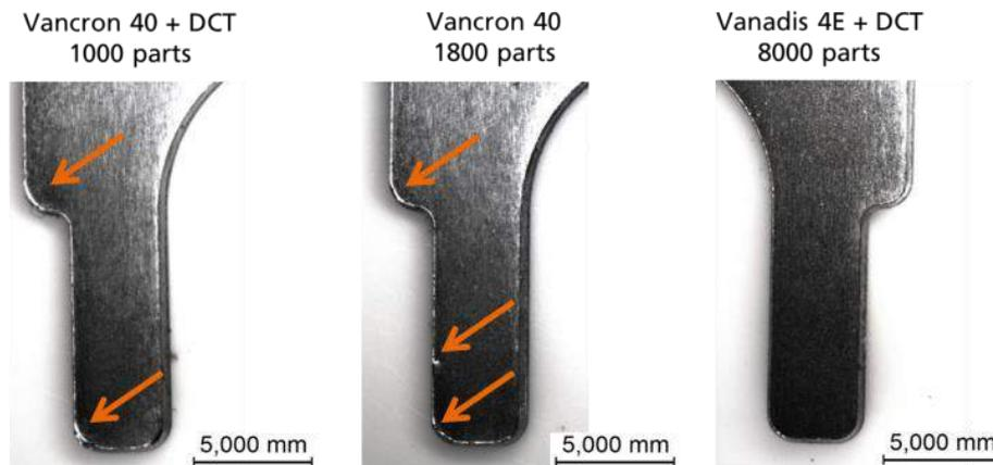
Figure 4-61: Critical burr formation at workpiece "gear folk" for different tool materials
