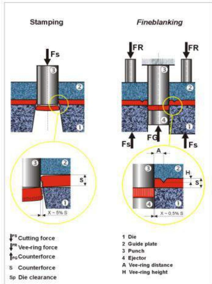
Figure 2-1: Differences between Cutting and Fine blanking
