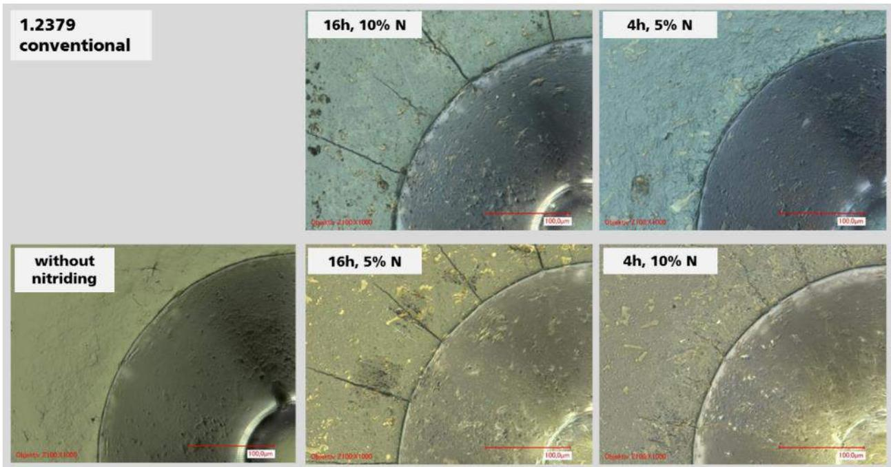
Figure 4-26: Crack resistance of 1.2379 with conventional heat treatment after plasmanitriding examined by Rockwell-indentation-test.
