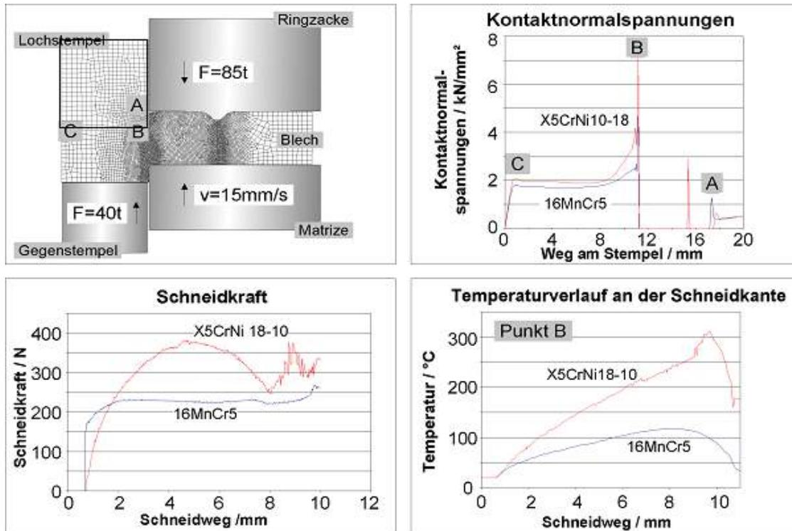
Figure 2-2: Calculation of the mechanical and thermal stresses of the tool for fine blanking of various materials. (Source: WZL, RWTH Aachen)
