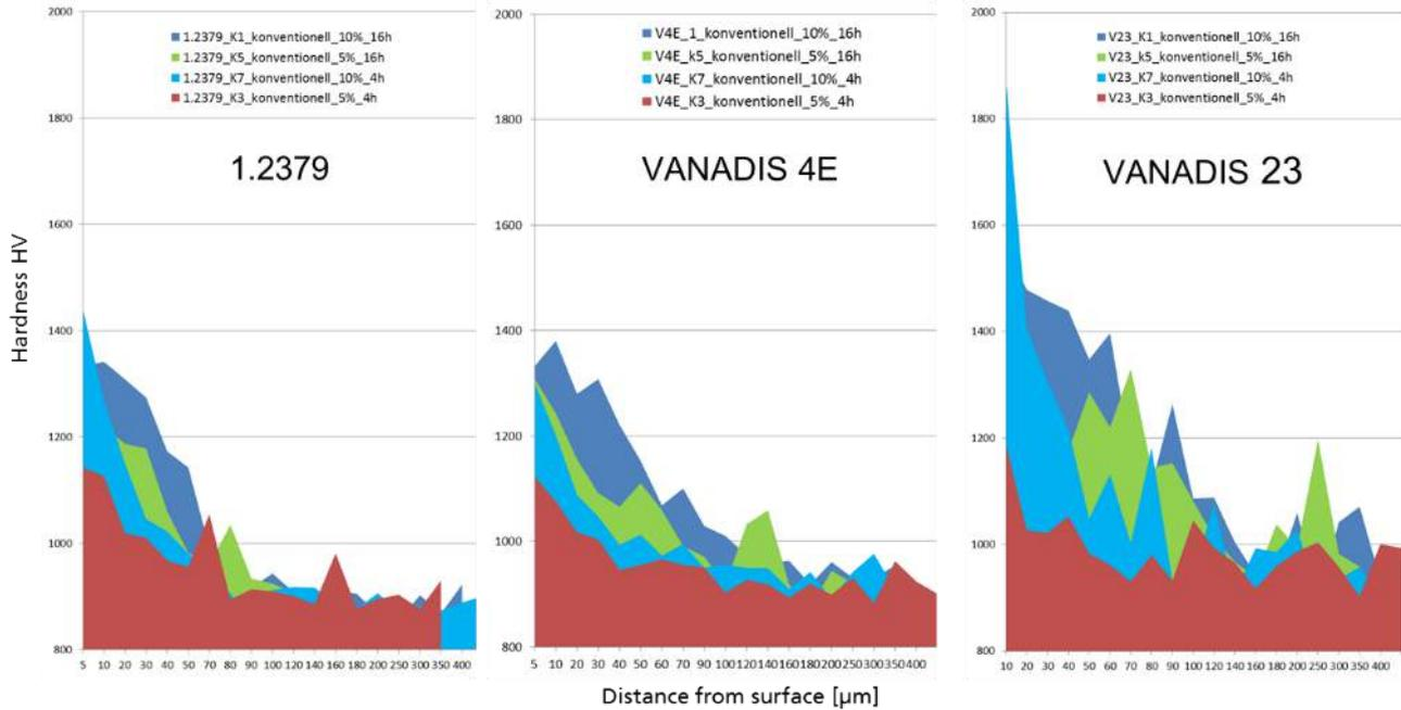
Figure 4-22: Hardness depth profiles in dependency on the nitriding parameters for conventional heat-treated 1.2379, Vanadis 4E and Vanadis 23
