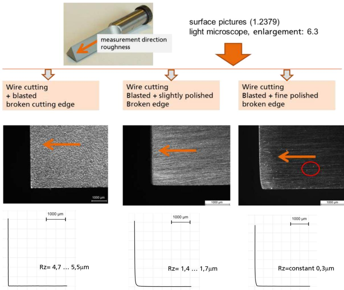
Figure 4-53: Manufacturing chain, surface topography, roughness and cutting edge of the tools for the lab scale tests
