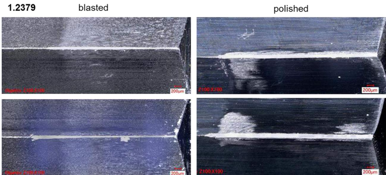
Figure 4-47: Adhesion on two edges of the tools made of 1.2379 with DCT treatment in dependency on the surface finishing after cutting stainless steel 1.4301 / 0,4 mm.
