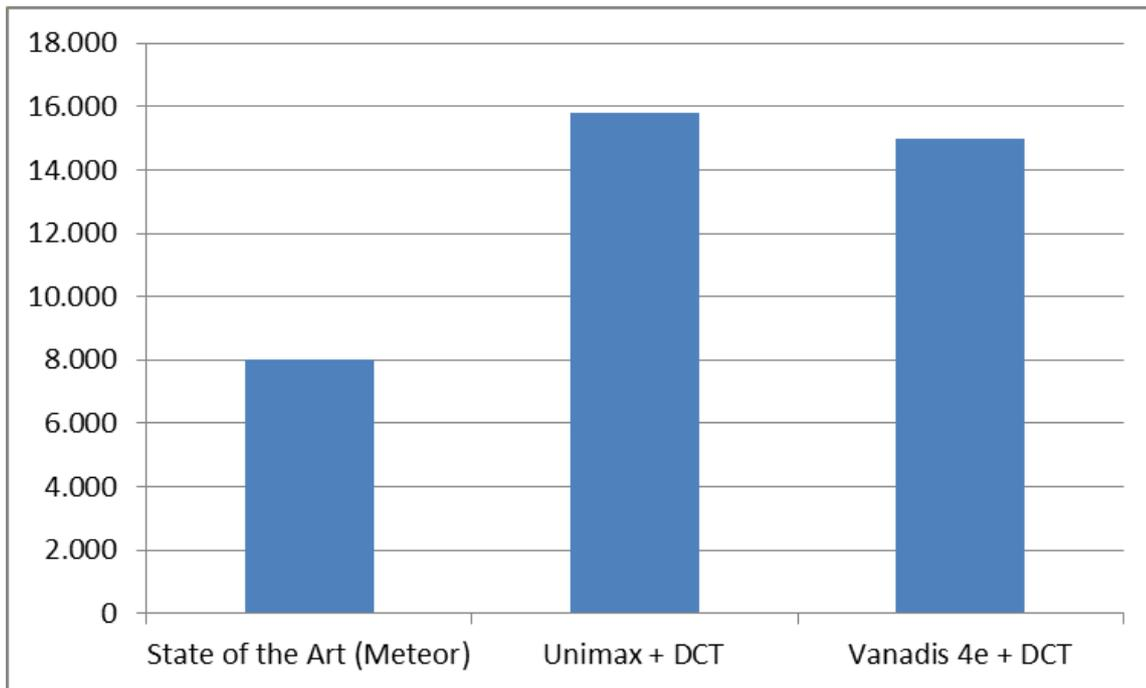
Figure 4-56: Overview of lifetime for industrial tests by company „Meteor“
