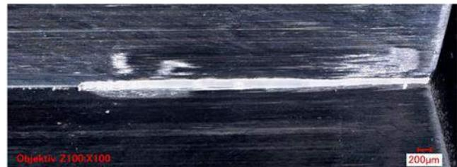
Figure 4-48: Adhesion on two edges of the tools made of Vanadis 4E and Vanadis 23 with DCT treatment in dependency on the surface finishing after cutting stainless steel 1.4301 / 0,4 mm.
