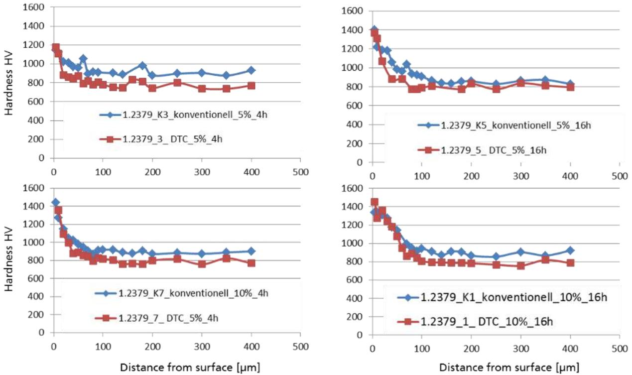
Figure 4-24: Hardness depth profiles in dependency on the nitriding parameters for conventional and DCT treated 1.2379
