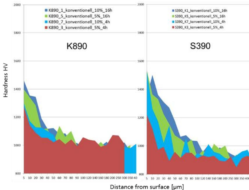
Figure 4-23: Hardness depth profiles in dependency on the nitriding parameters for conventional heat-treated K890 and S390
