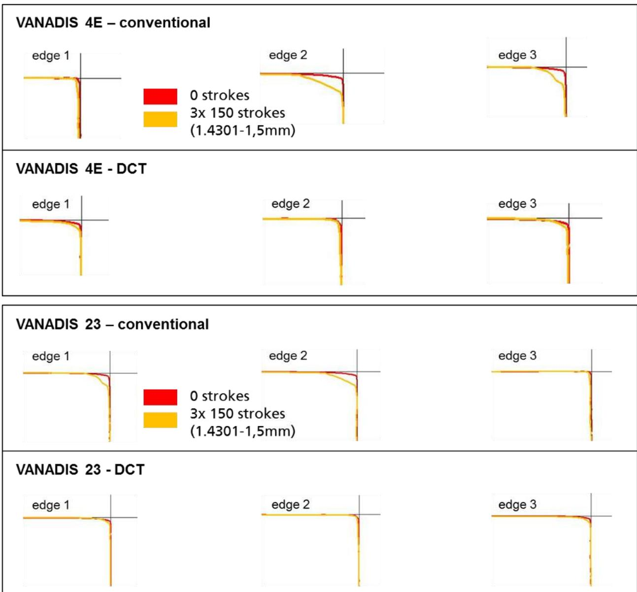
Figure 4-38: Wear measurement at the cutting edges of conventional and DCT treated Vanadis 4E and Vanadis 23 after cutting stainless steel 1.5 mm.
