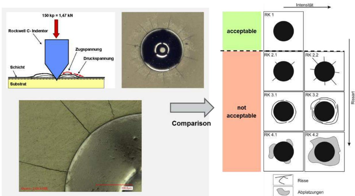
Figure 4-25: Examination of the nitriding result by Rockwell-indentation-test.
