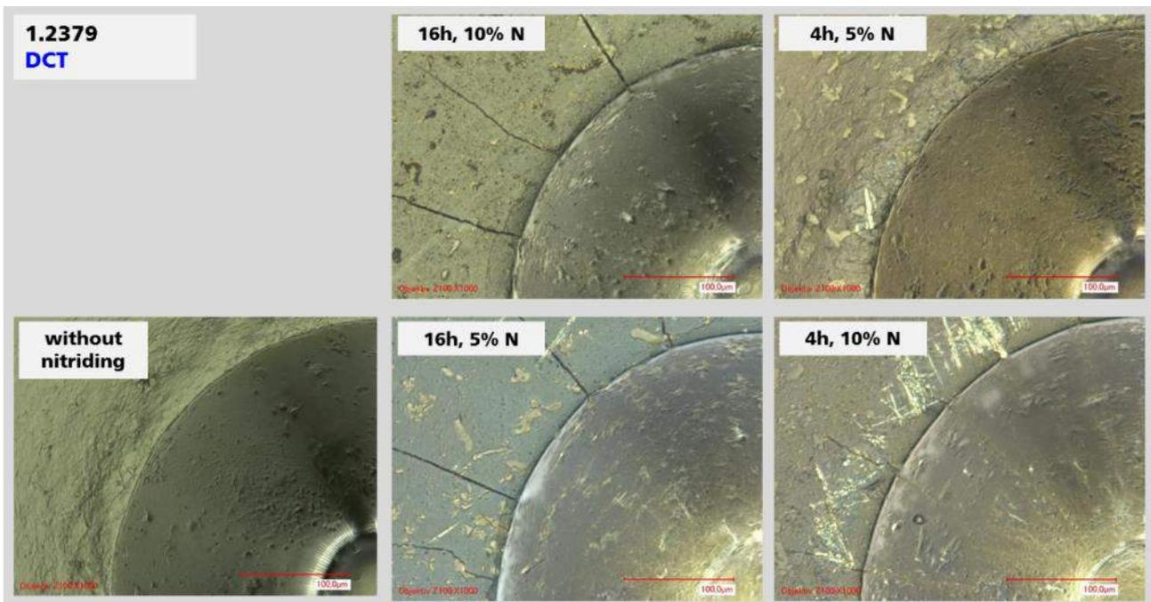
Figure 4-27: Crack resistance of 1.2379 with DCT after plasmanitriding examined by Rockwell-indentation-test.
