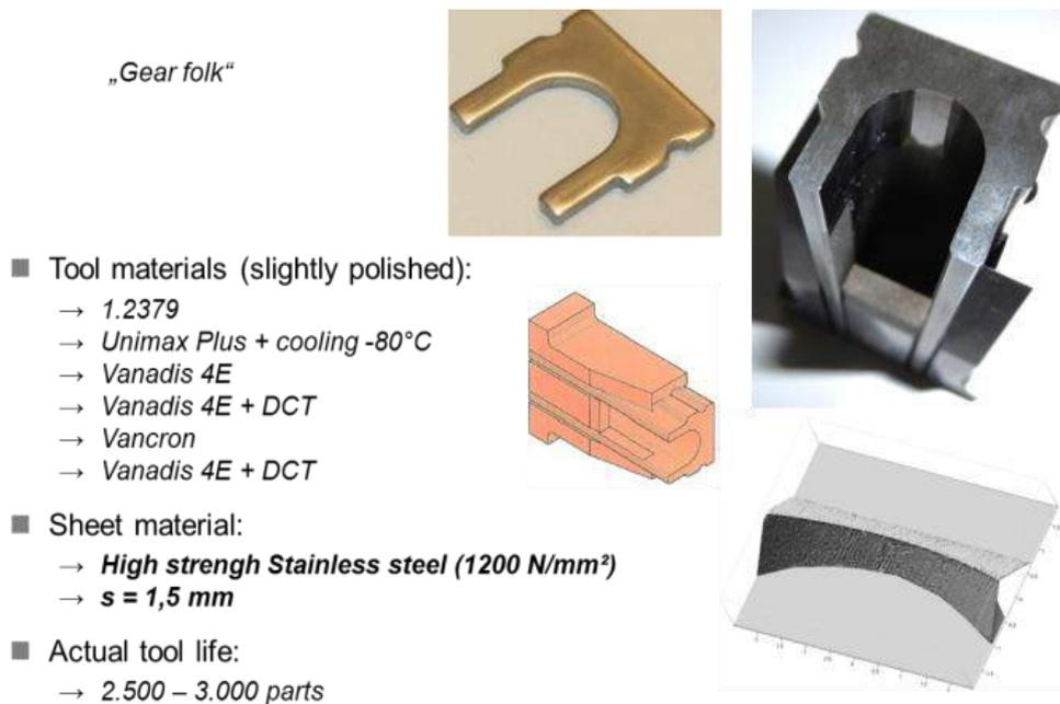
*Figure 4-57: Punch geometry, part geometry and test parameters of the blanking process at company “Karl Naumann GmbH”*
