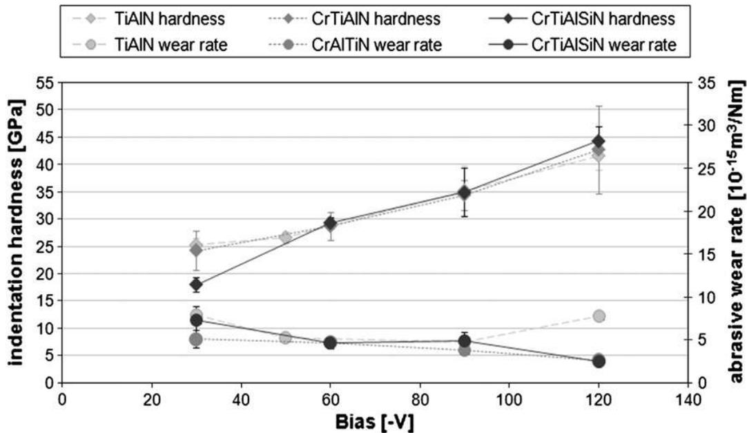
Figure 4-17: Coating hardness and abrasive wear rate vs. the applied substrate bias of Ti, Al and Si modified CrN coatings.
