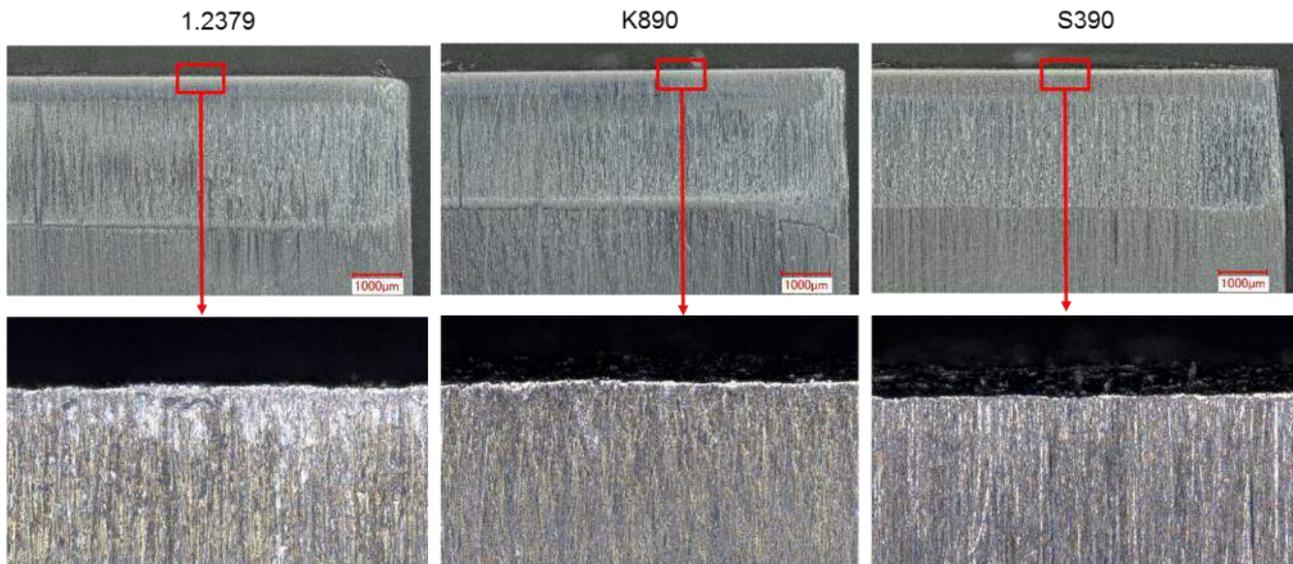
Figure 4-49: Wear at the cutting edges of the tools with DCT treatment and blasted and slightly polished surface after cutting DC04 / 1,5 mm.
