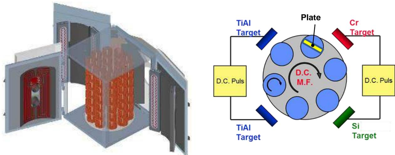
*Figure 4-13: Schematic illustration of the magnetron sputter machine CC800/9 from Cemecon.*
