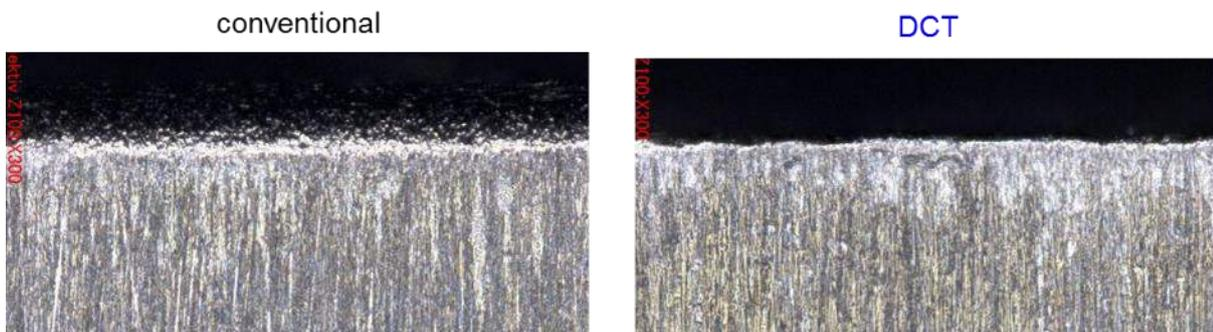
Figure 4-50: Wear at the cutting edges of 1.2379 (surface blasted and slightly polished) with conventional heat treatment and DCT treatment after cutting DC04 / 1,5 mm .
