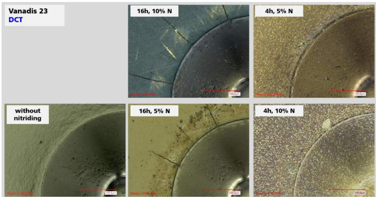
Figure 4-29: Crack resistance of Vanadis 23 with DCT after plasmanitriding examined by Rockwell-indentation-test.
