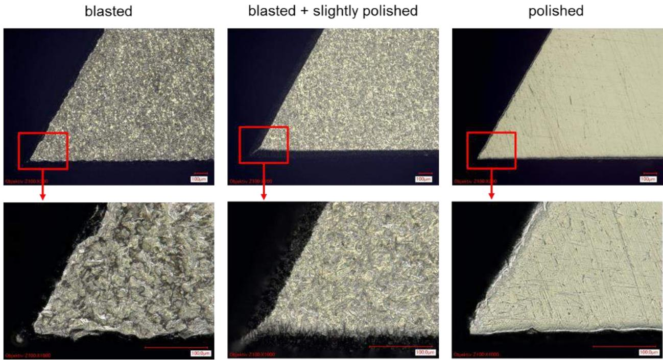
Figure 4-46: Surface finish at the cutting edges of 1.2379 before the cutting tests.
