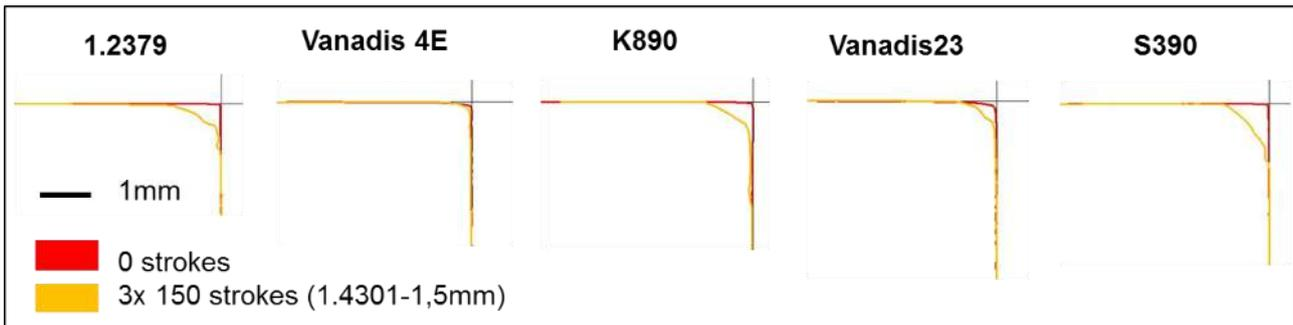
Figure 4-37: Wear measurement at the cutting edges of the conventional heat treated steels after cutting stainless steel 1.5 mm.
