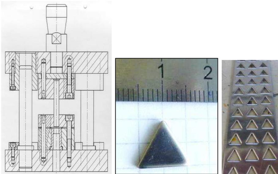
Figure 4-4: test tool at IWU Chemnitz/ size of cutted workpiece / cutted stripe-picture
