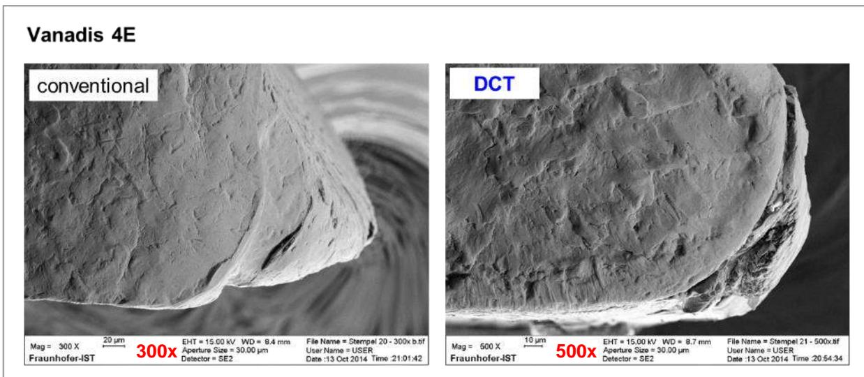
Figure 4-44: Comparison of the wear at the cutting edges of conventional and DCT treated 1.2379 and Vanadis 4E examined by SEM.
