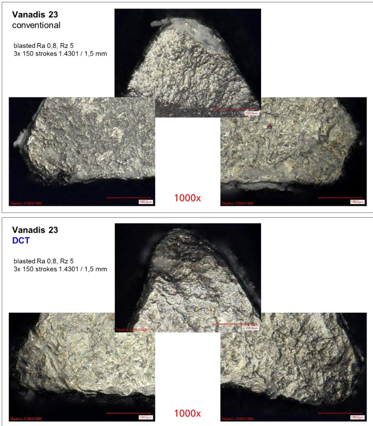
Figure 4-43: Comparison of the wear at the cutting edges of conventional and DCT treated Vanadis 23 examined by optical microscopy.
