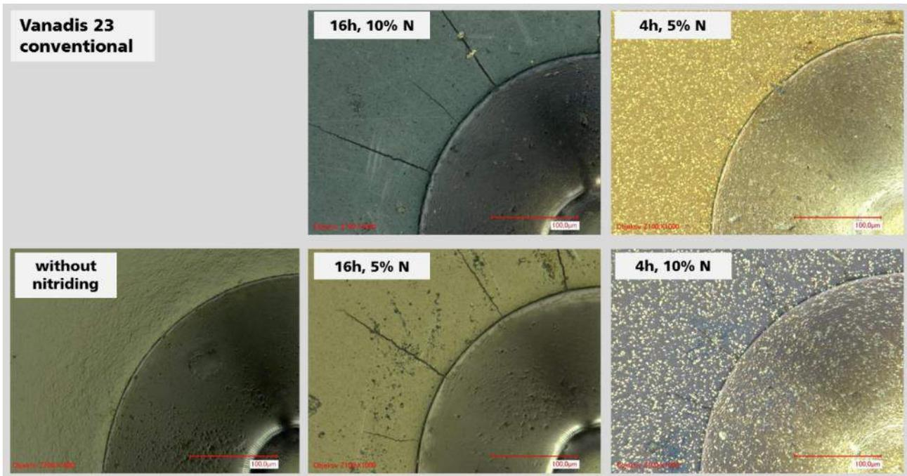
Figure 4-28: Crack resistance of Vanadis 23 with conventional heat treatment after plasmanitriding examined by Rockwell-indentation-test.
