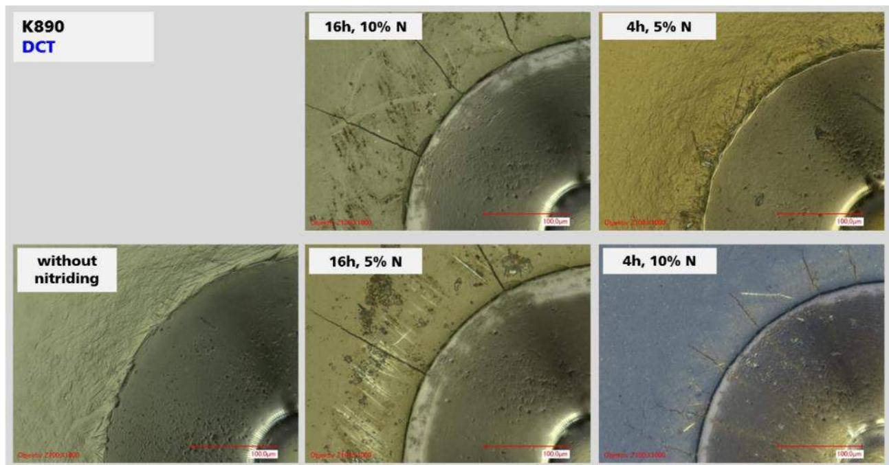
Figure 4-31: Crack resistance of K890 with DCT after plasmanitriding examined by Rockwell-indentation-test.
