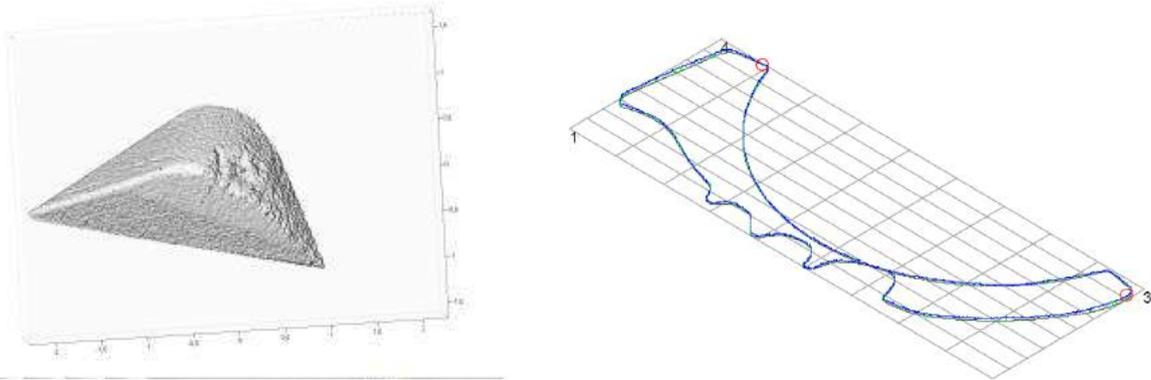
Figure 4-55: 3D-picture of the edge of the punch with abrasive wear (right) and a measurement of the tool contour (left)
