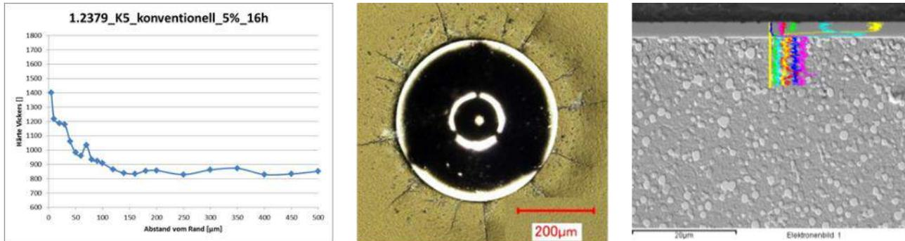
*Figure 4-21: Examples of the characterization of nitrided samples; (left) hardness depth profile, (middle) Rockwell-indentation with insufficient crack resistance, (right) SEM image and EDX analysis of a CrVN coated sample.*
