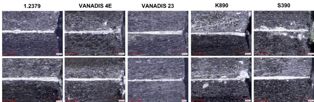
Figure 4-45: Wear at two edges of the tools with DCT treatment and blasted surface after cutting stainless steel 1.4301 / 0,4 mm..
