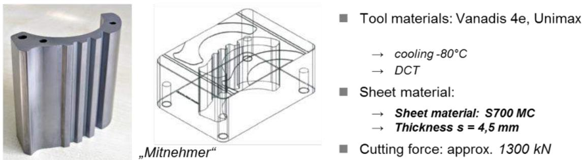
*Figure 4-54: Punch geometry and test parameters for the fine blanking process at company "Meteor"*
