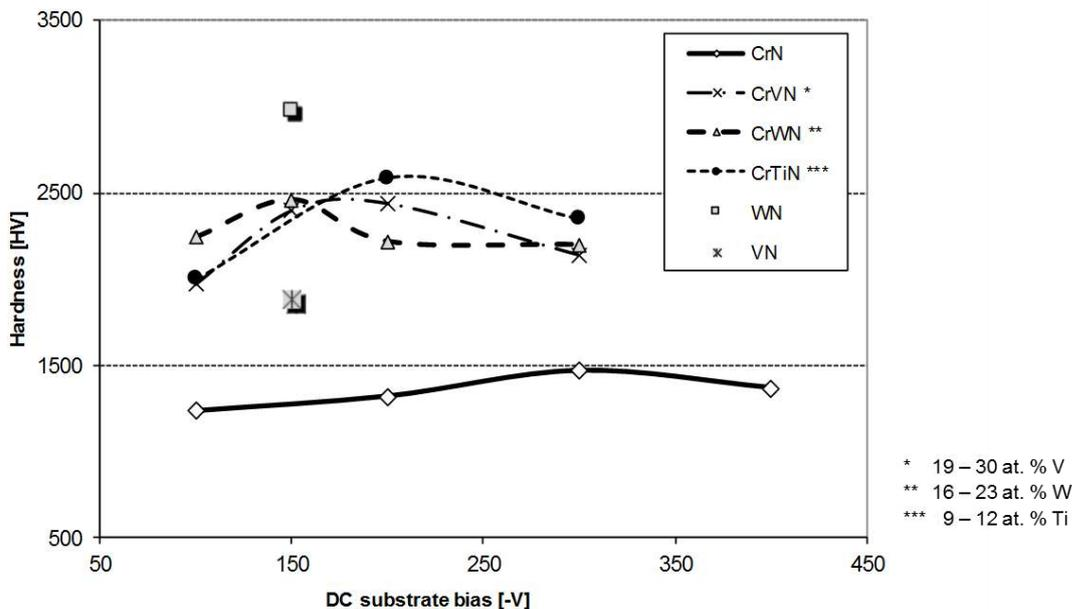
Figure 4-20: Coating hardness vs. the applied substrate bias of V, W and Ti-modified CrN coatings.
