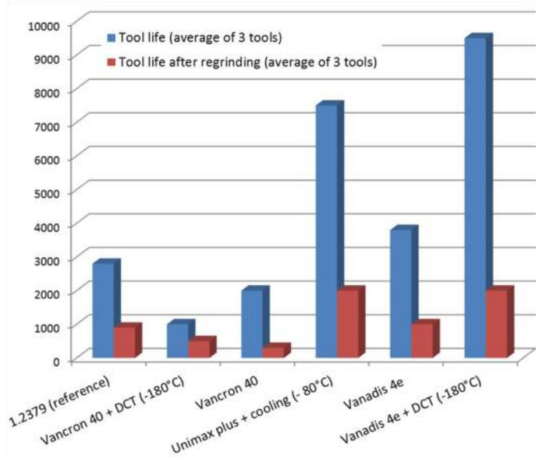
Figure 4-60: Tool life for different punch materials before and after first regrinding
