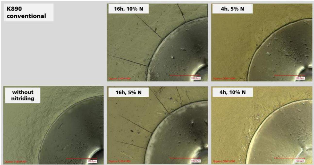
Figure 4-30: Crack resistance of K890 with conventional heat treatment after plasmanitriding examined by Rockwell-indentation-test.
