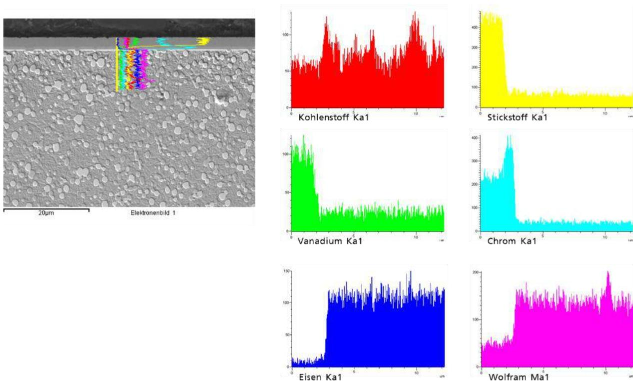
*Figure 4-33: SEM image and EDX analysis of a cross section of nitrided and CrVN coated S390 with conventional heat treatment (Cross section etched with Nital).*
