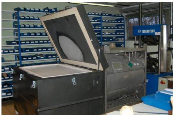
*Figure 4-8: Cryogenic chamber and liquid nitrogen tank for execution of DCT on materials*
