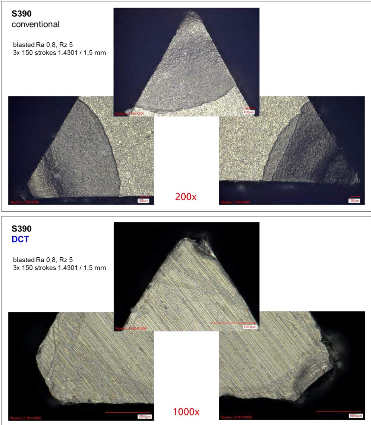
Figure 4-41: Comparison of the wear at the cutting edges of conventional and DCT treated S390 examined by optical microscopy.
