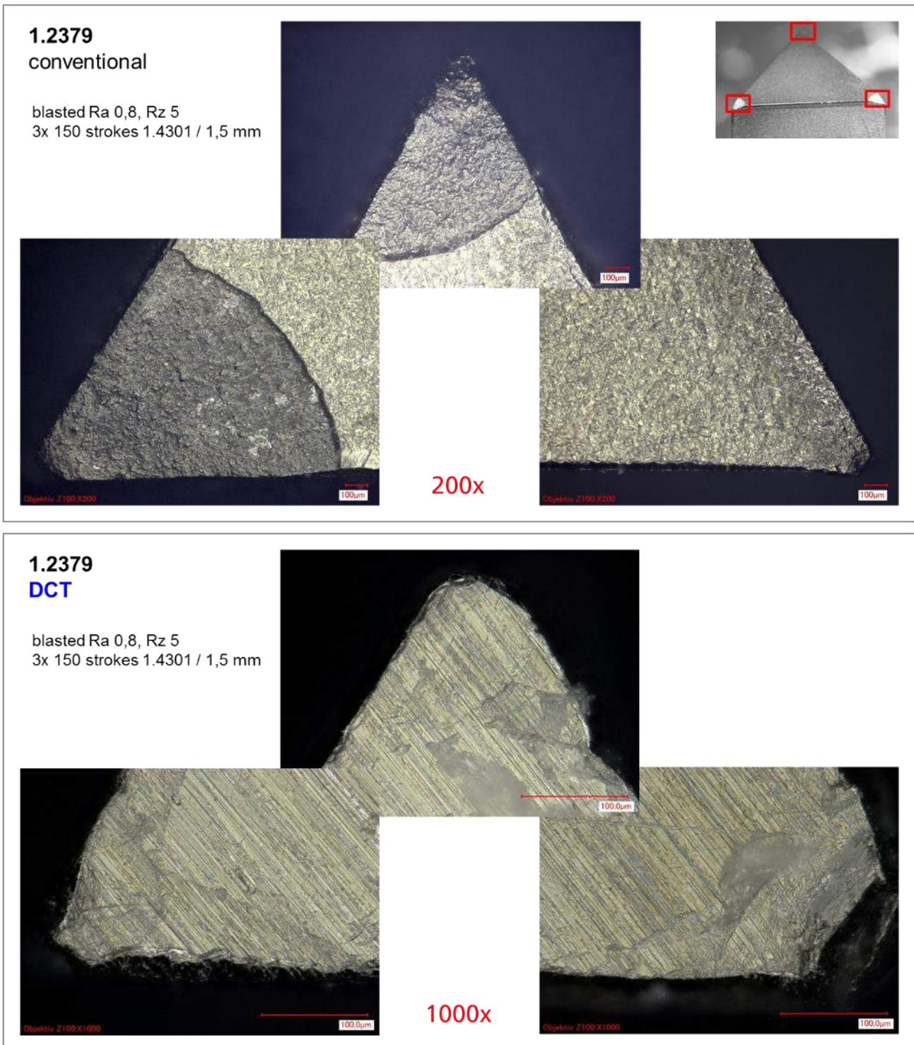
Figure 4-39: Comparison of the wear at the cutting edges of conventional and DCT treated 1.2379 examined by optical microscopy.
