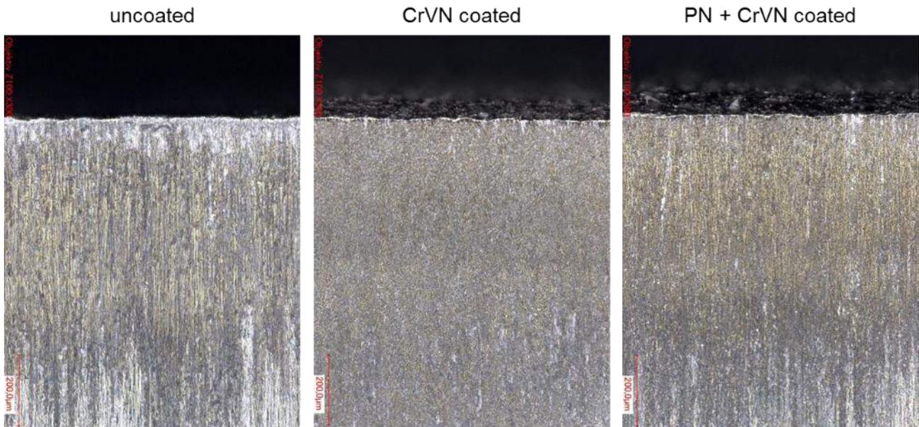
Figure 4-51: Adhesion on the cutting edges of DCT treated 1.2379 (blasted) with and without coatings after cutting DC04 / 1,5 mm.
