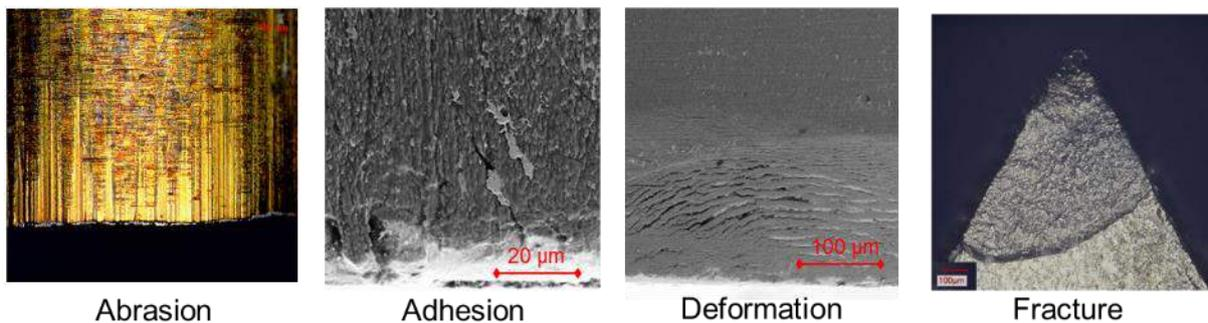
Figure 2-3: Wear mechanism on cutting tools. (Source: Fraunhofer IST, Fraunhofer IWU)
